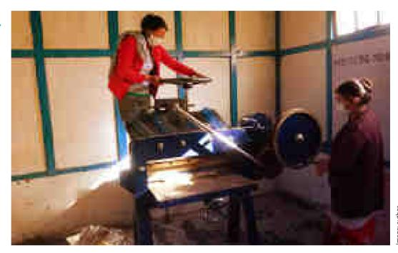
Local women artisans working on the pressing machine at the centre. The pressing machine squeezes out excess water from the pulp and makes it smooth
